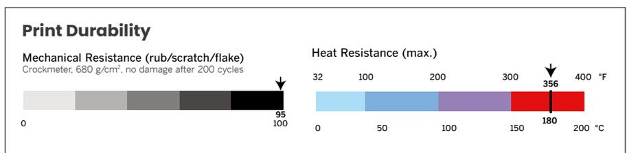
Videojet evaluation of observed performances of the Premium Ribbon with optimized printer setting and receptors.
